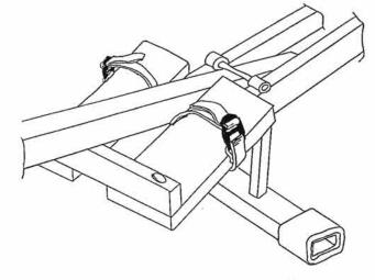
Note: If you have an older machine with screws, they will pass right through the footstrap. In newer machines with bolts, the strap will lie below the bolts.
