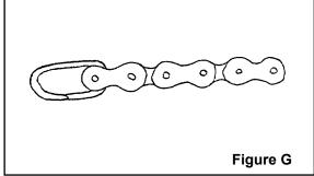
The end of the chain that connects to the front axle (dead end) will have one of three styles of connectors: 1) The fingered style as in Figure E. 2) A steel disc with holes in it as in Figure F. 3) A steel "lap-link" as in Figure G. All three of these connectors are reliable for this end of the chain.
