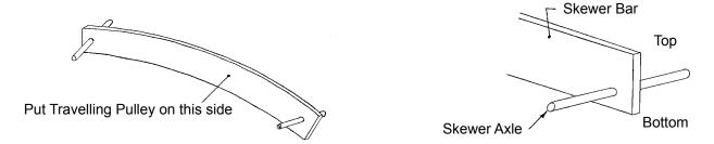
Figure B - Skewer Bar Bend Orientation (Exaggerated)
